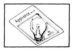
3. Replace the bulb only with a 40-watt appliance bulb from most hardware, grocery or variety stores.
