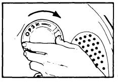
Open the dryer door and remove light bulb cover by turning it clockwise.
