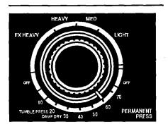
Select a cycle by turning the Cycle Control Knob either way. Stop when the indicator on the knob's outer ring points to the cycle and time you want. See pages 6-9 for further cycle information.
