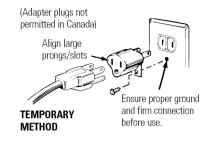
The larger slot in the adapter must be aligned with the larger slot in the wall receptacle to provide proper polarity in the connection of the power cord.
