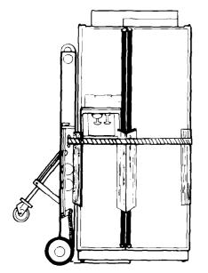
**3.** Place appliance dolly under the side of the refrigerator. Wrap strap from truck loosely around refrigerator. Insert two corner posts around handles to prevent scratching. Insert two corner posts over the cabinet side trim to prevent damage. Tighten strap making sure that handles and cabinet side trim will be protected.
