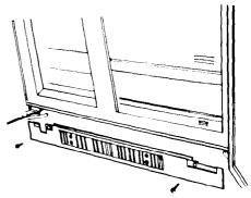
Open both doors. Use two screws to attach bottom grille to cabinet. Loosen the four height adjustment screws. Adjust the bottom grille to fill the space from the floor to the bottom of the cabinet. Tighten adjustment screws.
