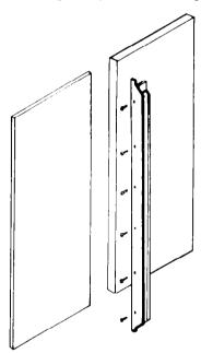
**10.** Remove all tape and door bracing from refrigerator door. Remove the six screws that attach the handle to the door frame. Slide the refrigerator door panel into door frame. If the panel is less than 1/4" thick, a filler panel will need to be installed between the door and decorative panel. If the decorative panel is more than 1/4" thick, it will have to be routed to have a 1/4" edge on all sides. See Custom panel and insert dimensions for exact sizes to cut custom panels.
