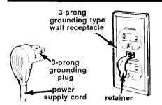
**5.** Move refrigerator close to final position. Remove cardboard or plywood from under refrigerator. Plug electrical cord into the grounded outlet. Use the screw from the parts package to install the plug retainer. Move the refrigerator evenly and straight into the opening. Check that the water line will not be kinked. Check that slack in the electrical cord hangs freely behind refrigerator or is placed on top of refrigerator next to cover.
