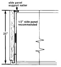
A side panel support nailer should be attached to the rear wall on each side of refrigerator when 25" depth is available. If less than 25" depth is available, go to step 3.
