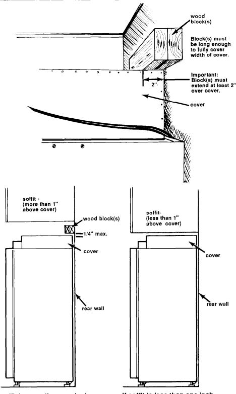
If soffit is more than one inch above cover, locate wall studs in the refrigerator opening. Center one wood block and use wood screws to attach the wood block to the wall studs. Make sure screws engage wall studs a minimum of 1-1/2". Screw the second wood block to the front of the first block. The wood block(s) must extend 2 inches beyond the ends of the cover.
