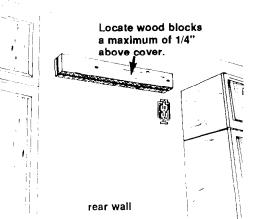
When a soffit is not available, locate wall studs in the refrigerator opening. Center one wood block and use wood screws to attach the wood block to the wall studs. Make sure screws engage wall studs a minimum of 1-1/2". Screw the second wood block to the front of the first block. The wood blocks must extend 2 inches beyond the ends of the cover.
