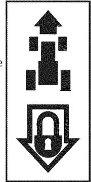
**NOTE:** Cruise control can NOT be engaged at the tractor's fastest ground speed. If the operator should attempt to do so, the tractor will automatically decelerate to the fastest optimal mowing ground speed.
