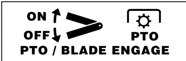
**NOTE:** The PTO (Blade Engage) lever must be in the disengaged (OFF) position when starting the engine, when traveling in reverse and if the operator leaves the seat.
