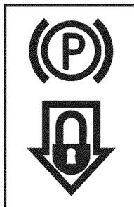
**NOTE:** The parking brake must be set if the operator leaves the seat with the engine running or the engine will automatically shut off.
