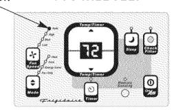
Note: The fan speed will begin in HI, then adjust to MED and LO as the room temperature conditions indictates. For example in cooling, if the room doesn't get too warm it will stay at LO. If the room temperature rises quickly, such as a door being opened, it will automatically go to HI speed. The fan speeds will adjust back to LO as the room returns to the original set temperature.
