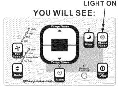
Note: This feature is a reminder to clean the Air Filter (See Care and Cleaning) for more efficient operation and cooling. The LED (light) will illuminate after 250 hours of operation. To reset after cleaning the filter, press the "Clean Filter" button and the light will go off.
