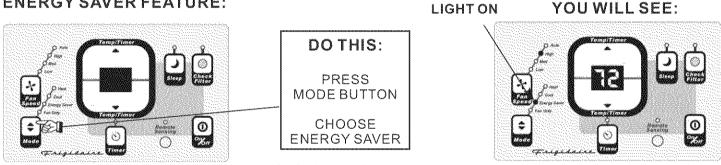
Note: In this mode, the fan will continue to run for 3 minutes after the compressor shuts off. The fan then cycles on for 2 minutes at 10 minute intervals until the room temperature is above the set temperature, at which time the unit cooling system starts again.
