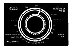
Select a cycle and time by turning the Cycle Control Knob either way to point to the cycle and time setting you want.
