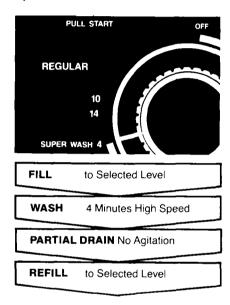
After the partial drain, the washer automatically refills and goes into the REGULAR Cycle. Be sure to use enough detergent for the double wash.
