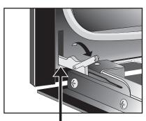
Lock engaged for door removal
