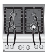
Your cooktop is equipped with different sized burners. The surface burners are located on the 30" models as follows (Fig. 1): a **5 000 BTU** (natural gas) burner at the right rear position; a **14 000 BTU** (natural gas) burner at the left rear position; and one **18 000 BTU Dual Flame** (natural gas) burner at the right and one **9 500 BTU** (natural gas) burner at the left front position.
