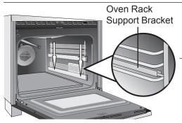
ALWAYS INSTALL OVEN RACK SUPPORT BEFORE TURNING ON THE OVEN (WHEN THE OVEN IS COOL). To remove the oven rack supports for a self-clean cycle,
