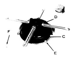
lower wash arm straight up. Lift filter out. TO RE-PLACE, clip outside filter over the inside filter and then replace wash arm. When replacing wash arm, be sure that water holes are facing up as shown in photo. If the outside filter needs frequent cleaning, or if there is foodsoil remaining on dishware, check underside of washarm for blockage of the single outside filter spray nozzle (G) or the nine inside filter spray nozzles (H). Clean out with a toothpick.
