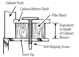
3 Attach the oven to the top cabinet by inserting 3 self-aligning screws through outer top cabinet holes. Turn two full turns on each screw. Be sure to keep power cord tight. Be careful not to pinch the cord, especially when mounting flush to bottom of cabinet.
