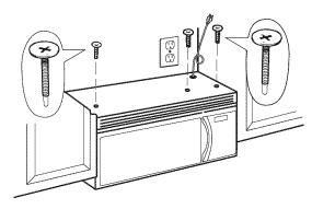
4 Tighten the three screws to the top of the oven completely. (While tightening screws, hold the oven in place against the wall and the top cabinet.)
