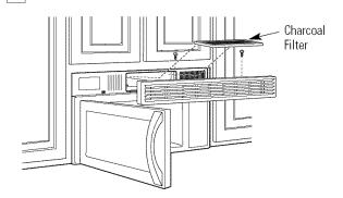
4 Insert the filter into the top of the opening, between the side support slots.
