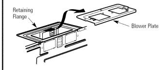
**3** Carefully pull out the blower unit. The wires will extend far enough to allow you to adjust the blower unit.
