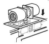
**6** Replace blower plate and replace screws for blower plate and blower motor removed in Step 1.
