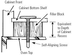
3 Attach the oven to the top cabinet by inserting 3 self-aligning screws through outer top cabinet holes. Turn two full turns on each screw. Be sure to keep power cord tight. Be careful not to pinch the cord, especially when mounting flush to bottom of cabinet.
