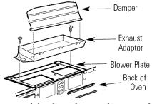
**NOTE:** On some models, the exhaust adaptor and damper assembly may already be assembled to the oven.
