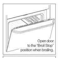
Always pull oven rack out to the "stop" position before turning or removing food.
