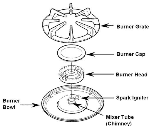
1. Place the Burner Head onto the Burner Bowl. Line the opening of the Burner Head with the location of the Spark Igniter.
