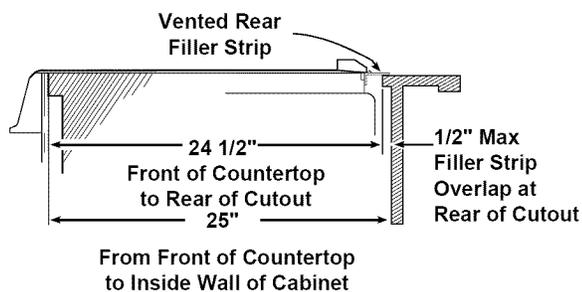
Use the screws provided to attach the filler strip to the back of the range.
