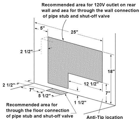
1. Install a manual shut-off valve in the gas supply line in an easily accessible location.
