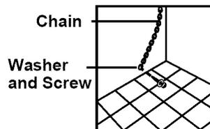
2. With the long screw provided anchor the chain to the floor or wall.
