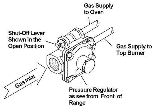
6. Install 1/2" flare union adaptor to the 1/2" NPT elbow on pressure regulator.
