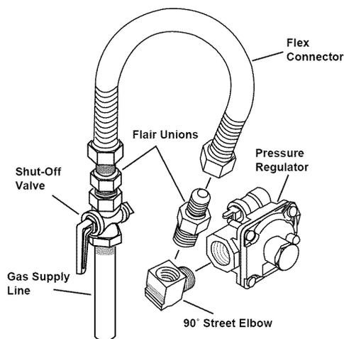
9. To prevent gas leaks, put a pipe joint sealant on all male threads.
