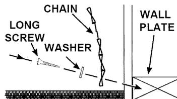
3. Make sure the screw is going into the wall plate or stud at the base of the wall at least 3/4".
