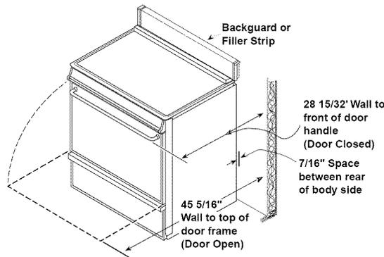
**▲** The cabinet must have solid sides, back, and bottom. The bottom must be solid either at floor level or with the bottom edge of the cutout. Any openings around the gas or electrical outlets must be sealed. All cabinet openings must be sealed at the time of installation to prevent drafts. Drafts will affect safe use of the oven.
