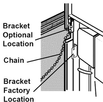
The upper set of holes are intended for use with an optional backsplash kit. If a backsplash kit is being used, the stability bracket can be relocated and put on the same time as the optional backsplash kit. If the backsplash is not being used, make sure that there are no countertop structural supports which will interfere with the stability bracket when located in the upper set of holes.
