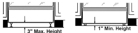
This gap is very important to the proper ventilation of the range and must be maintained when treating the appearance of the toe space.
