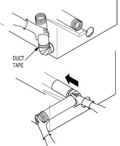
• Apply duct tape as shown on the joint between the dryer internal duct and the elbow.
