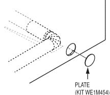
Connect standard metal elbows and ducts to complete the exhaust system. Cover back opening with a plate (Kit WE1M454) available from your local service provider. Place dryer in final location.
