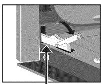
Lock engaged for door removal
