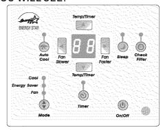
A 2 Digit Display is used to indicate the Fan Speed setting, from 10 through 99. When the "SLOW" button is pressed, the motor speed will slow down at multiple intervals (90 distinct settings), to a minimum setting of 10. To speed the motor up, press the "FASTER" button. The speed will increase at multiple intervals to a maximum setting of 99. After 5 seconds the control will automatically change back to displaying the set temperature.
