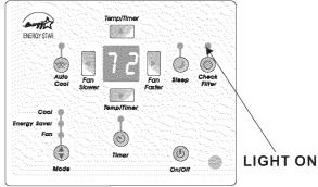
NOTE: This feature is a reminder to clean the Air Filter (See Care and Cleaning) for more efficient operation. The LED (light) will illuminate after 250 hours of operation. To reset after cleaning the filter, press the "Check Filter" button and the light will go off.
