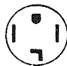
TYPICAL 4 CONDUCTOR RECEPTACLE
