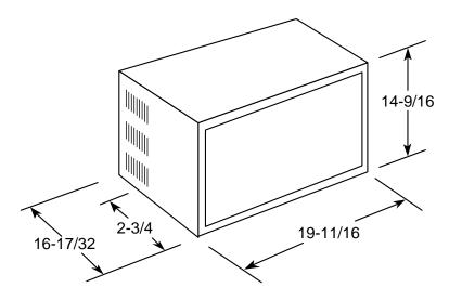
Note: When installing units in through-the-wall applications, keep louvers free. Do not restrict air flow areas. Carry-Cool® units are not designed for through-the-wall applications.
