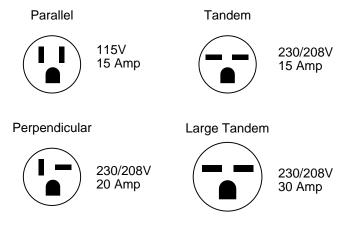
Wall Outlets: All wiring including installation of receptacle must be made in accordance with local electrical codes and regulations. Electrical outlet should be in reach of line cord.
