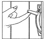
Set the control lever to VEG to convert the drawer to normal
