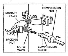
6. Slip compression sleeve and compression nut on copper tubing as shown above. Insert end of tubing into outlet end squarely as far as it will go. Screw compression nut to outlet end with adjustable wrench. Do not overtighten. Turn ON main water supply and flush out tubing until water is clear. Turn OFF shutoff valve on water pipe. You are now ready to connect other end of 1/4" copper tubing to water valve on back of refrigerator.
