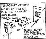
**CAUTION:** Attaching an adapter ground terminal to the wall outlet cover screw does not ground the appliance unless the cover screw is metal, and not insulated, and the wall outlet is grounded through the house wiring. You should have circuit checked by a qualified electrician to make sure the outlet is properly grounded.
