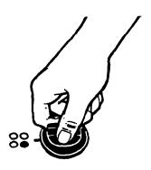
2. Line up openings in the reflector bowl with the surface unit receptacle and the element hold-down clip.
