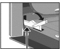
Lock engaged for door removal
