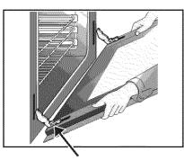
HINGESLOT-Doorremoved from the appliance
