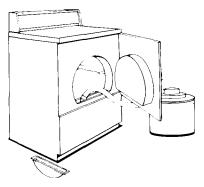
Do not obstruct the flow of combustion and ventilating air. The air intake is located on rear of dryer.
