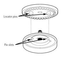
When placing, make sure the locator pins in the burner head are seated in the pin slots of the burner base. Rotate the burner head around the burner base until it is level and securely seated.
