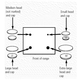
Replace the burner heads on the bases matching the letters. Replace the caps on the heads. Make sure that the caps and heads are replaced in the correct location. There is one small, one medium, one large and one extra large head and cap.
