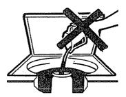
Do not pour anything into the agitator if the agitator cap or dispenser is removed.
