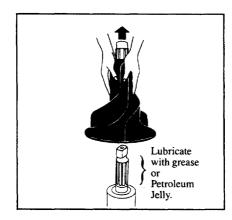
The Activator® agitator. Remove at regular intervals—about 4 to 6 months—and remove any lint that may have accumulated. No tools are needed, simply grasp agitator with both hands and pull straight up sharply. The slotted section at the top of the metal shaft has a light coating of lubricant to prevent parts sticking together. If this area appears to be dry, apply a light coat of grease or petroleum jelly around the slotted section of the shaft before replacing the agitator. Do not overgrease.
