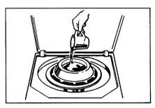
7. Add fabric softener, if desired. Place the Fabric Softener Dispenser on the Filter-Flo pan. Pour 1 teaspoon (5 ml) of concentrated softener or 1 tablespoon (15 ml) of diluted softener into a standard measuring cup. Add enough water to fill the cup 1/2 full. Pour the diluted softener into the dispenser. See page 9 for dispenser instructions.
