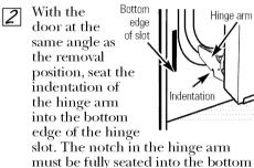
of the slot. Fully open the door. If the door will 3 not fully open, the indentation is not seated correctly in the bottom edge of the slot.
