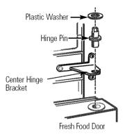
Remove the tape and tilt the door away from the cabinet. Remove and save the washer on the hinge pin. Lift the door straight up to free its bottom socket from the pin in the bottom hinge bracket.
