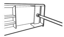
Replace the base grille by inserting the tops of the metal clips into the oval vents, making sure one of the plastic tabs on the back of the grille goes into each of the oven vents. Then push the bottom of the grille forward until it snaps into place.
