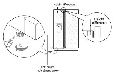
If the freezer compartment door is higher than the refrigerator compartment door Level the door by inserting flat ( - type) driver into the groove of the right height adjusting screw and rotate it clockwise  $(\mathbb{O})$ .
