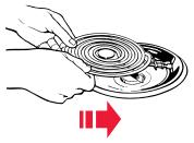
Hold the surface unit as level as possible with the terminal just started into the receptacle. Push the surface unit terminal into the receptacle.
