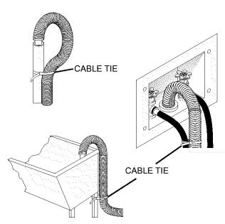
7. Form a "U" shape on the end of the drain hose with the hose pointed toward the drain. On some models, a wire retainer needs to be assembled on the hose in that position. Place the formed end in a laundry tub or a standpipe and secure with a cable tie provided in the enclosure package.
