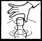
DO NOT add or remove anything while the washer is agitating or spinning. If the washer lid is opened during the spin, the washer will automatically stop in a few seconds.
