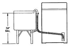
When water faucets and standpipe are built into the wall, secure the drain hose with the shipping strap as follows:
