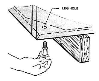
Remove the wood block and gently lower the washer to the floor.
