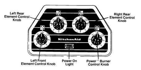
The white circle in the diagram above each knob indicates which element that particular knob controls.
