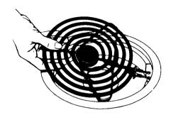
Guide the element into the receptacle opening. Push element all the way forward so it fits snugly in the receptacle. To make sure element sits flat, place palm of hand flat on top of element and exert a slight downward force.
