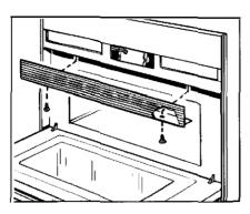
Step 3: Rotate the light bulb housing out and toward you to access the light bulb. Replace the burned-out bulb with a 40-watt incandescent bulb (WB02X4253)
