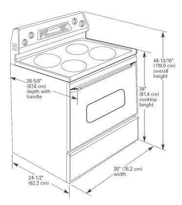
When installed in a 24" (61.0 cm) base cabinet with 25" (63.5 cm) countertop, front of oven door protrudes 1-7/8" (4.8 cm) beyond 24" (61.0 cm) base cabinet.
