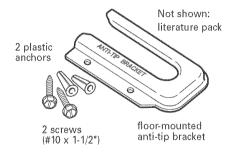
Brackets must be securely mounted to sub-floor. Thickness of flooring may require longer screws to anchor bracket to sub-floor. Longer screws are available from your local hardware store.
