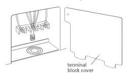
Depending on your electrical supply, make the four-wire or three-wire connection to the range following the "Power supply cord method" or "Direct wire method" instructions for copper wire or aluminum wire depending on the connection needed.
