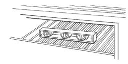
If range is not level, pull range forward until rear leveling leg is removed from the anti-tip bracket. Use 3/8" drive ratchet and channel lock pliers to adjust leveling legs up or down until range is level. Push range back into position. Check that rear leveling leg is engaged in anti-tip bracket.
