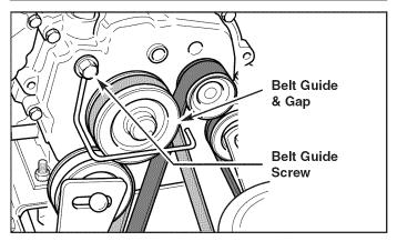
Figure 28. Auger Belt Guide Adjustment
