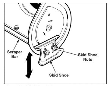
Figure 10. Skid Shoe Adjustment
