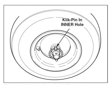
Figure 12. Traction Drive Lock - Engaged
