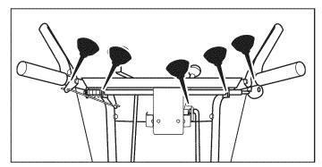
Figure 17. Lubricate Free Hand Control
