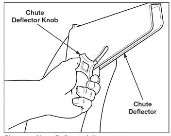
Figure 9. Chute Deflector Adjustment
