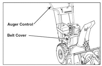
Figure 25. Auger Control and Belt Cover Location
