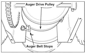
Figure 30. Auger Drive Pulley and Belt Stops
