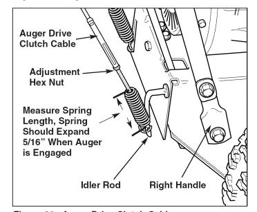
Figure 26. Auger Drive Clutch Cable
