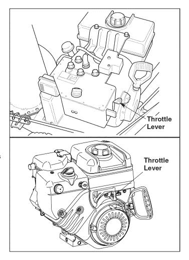
Figure 8. Engine Speed Selection
