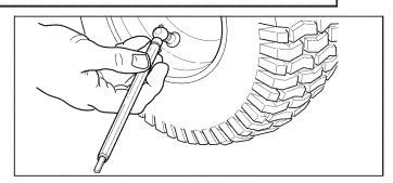
Figure 13. Checking Tire Pressure
