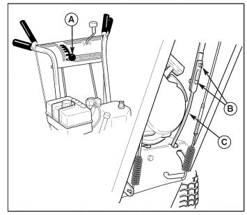
Figure 19. Speed Selector Linkage Adjustment
