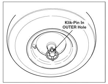
Figure 11. Traction Drive Lock - Disengaged
