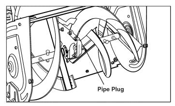
Figure 14. Checking Auger Gear Case Lubrication
