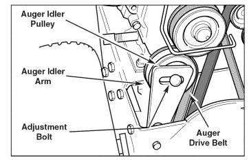
Figure 27. Auger Drive Belt, Guide and Pulley
