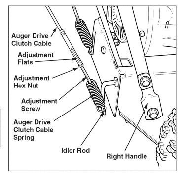
Figure 23. Auger Drive Clutch Cable Adjustment
