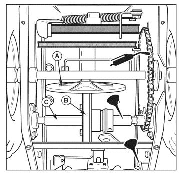
Figure 15. Drive Area Lubrication Points (Bottom Cover Removed)
