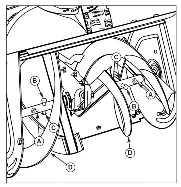
Figure 18. Checking Auger Gear Case Lubrication
