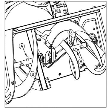
Figure 32. Shear Pin Replacement A. Shear Pin B. Cotter Pin
