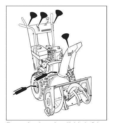
Figure 16. Snowthrower General Lubrication Points
