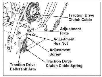
Figure 20. Traction Drive Clutch Cable Adjustment
