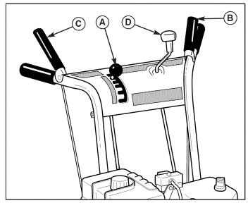
Figure 3. Operator's Control Position A. Speed Selector
