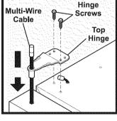
**4** Remove the screws from the top hinge and pull the multi-wire cable through it. Lift the door off of the bottom hinge.
