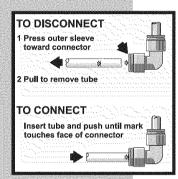
3 Detach the water tube from the connector located below the freezer door. The connector releases when you press its outer sleeve inward.
