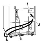
1. Cold water inlet valve (blue) 2. Hot water inlet valve (red)
