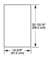
A 7/32" (5.6 mm) thick panel is required. This is the same thickness as a standard 1/4" plywood or paneling.
