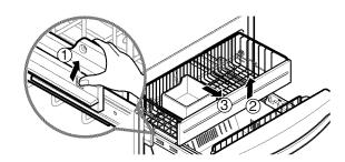
To install, reposition the gear part of rear left and right side of the drawer after pulling out both rails as much as possible, and gently push down both left and right side while checking the hook on the front part.
