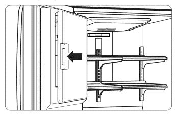
2. To remove the in-door ice bank, grip the front handle, slightly lift the lower part, and slowly pull out the bin as shown.
