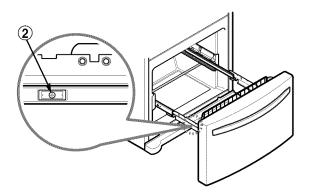
• With both hands, hold both sides of the door and pull it up to separate it from the rails.
