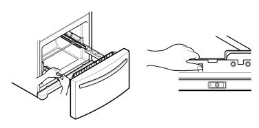
• Remove the screws(2) of the rail on both sides.
