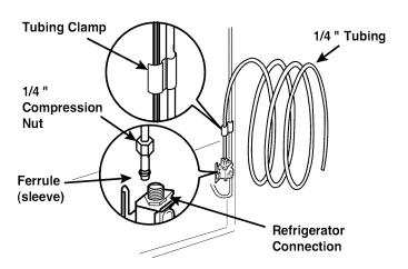
▲ CAUTION: Check to see if water dripping occurs at water line connections.
