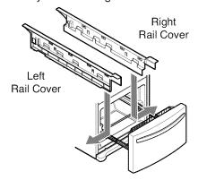
• Align the top holes of the rail cover with the top holes of the door supports to assemble the rail covers.
