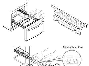
• With the drawer pulled out to full extension, insert the lower basket (4) in the rail assembly.
