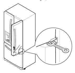
Level the refrigerator by using an 11/16 inch (18mm) wrench or a flat blade screw driver.
