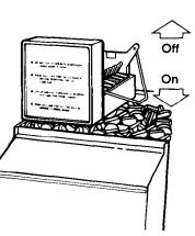
For crushed ice, cubes are crushed before being dispensed. This may cause a slight delay when dispensing crushed ice. Noise from the ice crusher is normal, and pieces of ice may vary in size.
