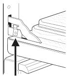
LOCK ENGAGED FOR DOOR REMOVAL
