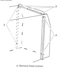
2. Insert cabinet into the framed wall opening. The top of the cabinet should extend <sup>3</sup>/<sub>4</sub> (19.1 mm) into the room. If there is trim, the cabinet should extend <sup>3</sup>/<sub>4</sub> (19.1 mm) past the trim.
