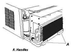
NOTE: Do not lift, push, pull or remove any expanded polystyrene (foam) from inside the air conditioner. It is not packing material.
