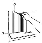
A. #10 x ¾" round-head screw B. Slotted hole in the bottom of the curtain
