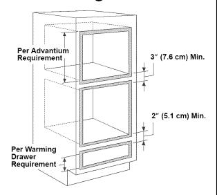
**NOTE:** The middle rail separating the two openings may need to be larger than the 3" (7.6 cm) minimum shown. Always refer to the individual installation instructions packed with each product for specific requirements.
