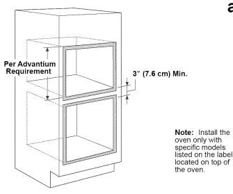
**NOTE:** The middle rail separating the two openings may need to be larger than the 3" (7.6 cm) minimum shown. Always refer to the individual installation instructions packed with each product for specific requirements.
