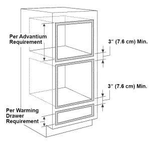
NOTE: Additional clearances may be required. Check to be sure the oven supports above the Warming Drawer do not obstruct the required interior depth and height. The middle rail separating the openings may need to be larger than the 3" (7.6 cm) minimum shown. Always refer to the individual installation instructions packed with each product for specific requirements.
