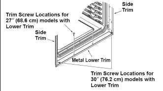
IMPORTANT: If this unit is ever removed from the cabinet or the oven is ever pulled out for service, the trim must be removed first or damage to the trim will occur.
