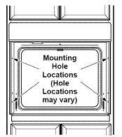
The screws must be a minimum of 1/4" (6 mm) from the front of the cutout.
