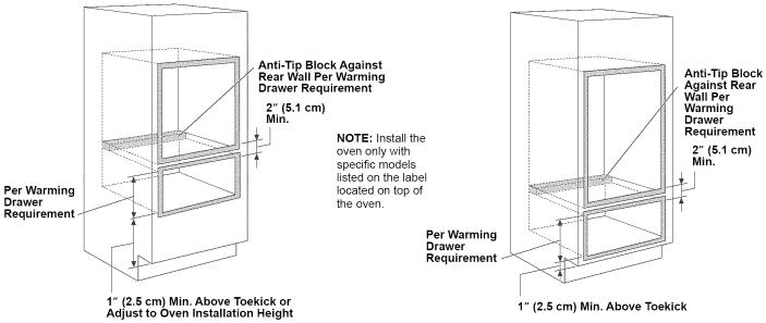
**NOTE:** Additional clearances between cutouts may be required. Check to be sure the oven supports above the Warming Drawer location do not obstruct the required interior depth and height.
