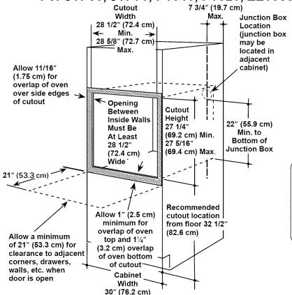
NOTE: If the cabinet does not have a front frame and the sides are less than 3/4" (1.9 cm) thick, shim both sides equally to establish the cutout width.
