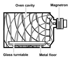
The glass turntable of your microwave oven lets microwaves pass through. Then they bounce off a metal floor, back through the glass turntable, and are absorbed by the food.
