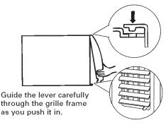
Press the grille frame in around the power cord on the right side. Secure the grille with a type F (painted) screw on each side and a type C screw in the front.
