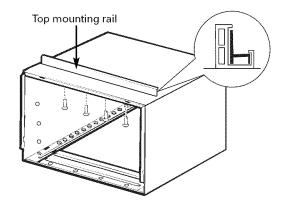
Insert the frames for the accordion panels into the top mounting rail and the bottom frame guides. Attach the accordion panels to the side of the case using 3 type A screws on each side.
