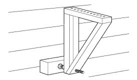
Adjust the leveling bolts and nuts against the outside wall so that the case has a slight tilt to the outside. Tighten nuts with an adjustable wrench. Use a level; about a 1/2 bubble will be the correct case slant to the outside.
