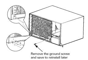
Slide the air conditioner from the case by gripping the base pan handle and pulling forward while bracing the case.
