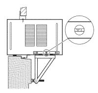
Extend the left and right accordion panels to the vertical window sashes. Drill pilot holes and attach the top and bottom corners with 4 type D screws.
