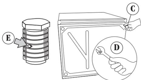
Start to screw legs (C) into holes by hand. Use an adjustable wrench (D) or 1" hex-head socket wrench to finish turning legs until you reach the ridge with the diamond marking (E).
