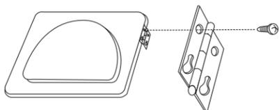
Attach door hinge to door so large part of hinge slot is at bottom of hinge.
