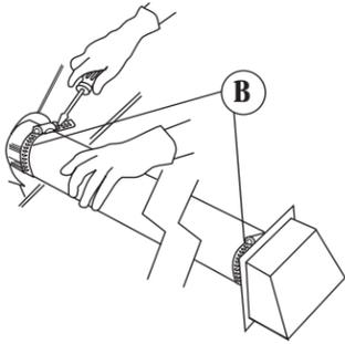
Using a 10.2-cm (4 inch) clamp (B), connect exhaust vent to exhaust outlet in dryer. If connecting to existing exhaust vent, make sure the vent is clean. The dryer exhaust vent must fit over the dryer exhaust outlet and inside the exhaust hood.
