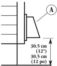
**Exhaust outlet hood** must be at least 30.5 cm (12 inches) from the ground or any object that may be in the path of the exhaust (such as flowers, rocks or bushes, etc.).
