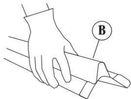
Take two cardboard corners (B) from dryer carton and place them on floor in back of dryer. Firmly grasp body of dryer and gently lay it on its back on the cardboard corners.
