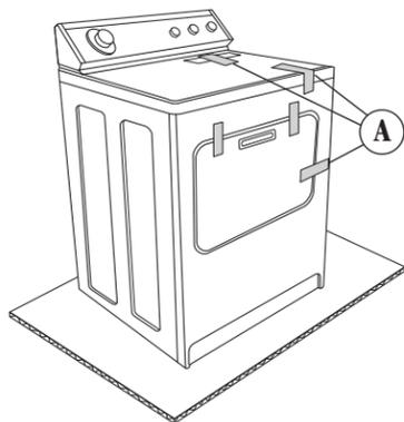
Remove tape (A) from dryer cabinet. Open dryer door and remove tape from dryer drum. (Not all dryer drums are taped.) Remove drying rack, if included. Turn dryer drum counterclockwise to make sure all tape was removed. Wipe drum with damp cloth to remove any dust.
