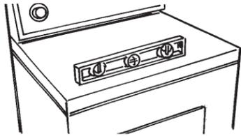
Check levelness of dryer by placing a level on top of dryer, first side to side, then front to back. If dryer is not level, adjust dryer legs up or down.
