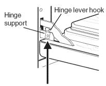
Lock engaged for door removal Figure 1
