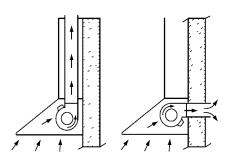
To prevent a back draft, never decrease the duct size over the run If existing duct work is smaller than 8 inches in diameter, remove it and replace it with 8" round, 10" inch round or 3 1/4" x 10" duct work Do not use duct work that is smaller in cross-sectional area than these recommended types Do not use flexible metal duct
