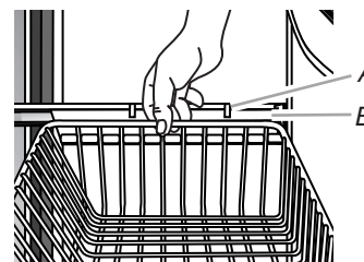
A. Cradle snap attachment B. Basket cradle
