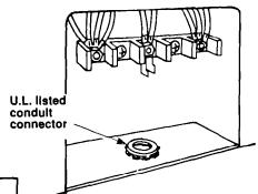
If appliance is to be connected directly to fused disconnect or circuit breaker **box:** Assemble a U.L.-listed conduit connector in the conduit connector opening provided. Insert the power supply cable through the conduit connector. allowing enough slack to easily attach the wiring to the terminal block.
