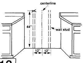
To mount anti-tip bracket to wood L or metal wall stud: Find the wall stud that is closest to the center of the range location. (Note: Wall stud should Not be more than 12 inches to the right or left of center of range location.) Measure and mark at the center of the wall stud a distance of 44 inches up from the floor.
