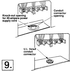
If appliance is to be connected directly to fused disconnect or circuit breaker box: Assemble a U.L.-listed conduit connector in the conduit connector opening provided. Insert the power supply cable through the conduit connector, allowing enough slack to easily attach the wiring to the terminal block.
