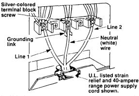
If a U.L.-listed, 40-ampere range power supply cord (pigtail) is used: Remove the knockout for the 40-ampere power supply cord.
